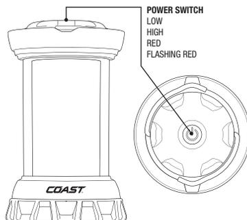
Depressing the same button a second time will switch the lantern to "high" white LED Power mode. A third depression of the button will turn the lantern into "solid" red LED mode. A fourth depression of the button will turn the lantern into "flashing" red LED mode. To turn off the lantern, depress the power switch a fifth and final time.
